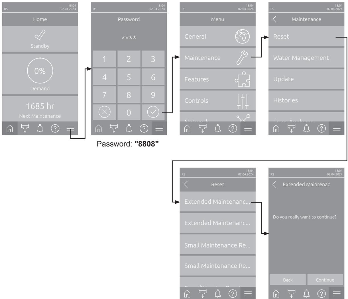
1. Select in the "Reset" submenu (Path: "Menu > Password: 8808 > Maintenance > Reset"). Then select the corresponding reset function ("Extended Maintenance Cyl. A Reset", "Extended Maintenance Cyl. A Reset" "Small Maintenance Cyl. A Reset" or "Small Maintenance Cyl. A Reset").
