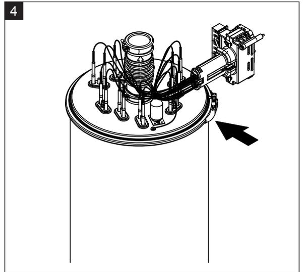
4. Undo the steam cylinder cover clamping ring.
