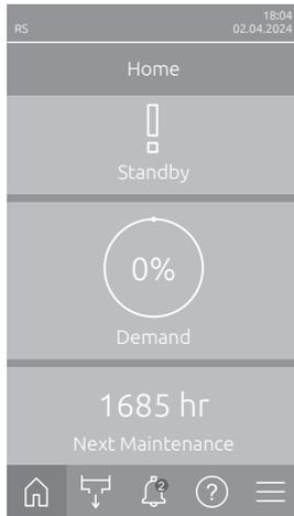
Temporary problems (e.g., water supply interrupted for a short time) or malfunctions which cannot cause damage to the system are indicated with a warning message, additionally the status LED lights up yellow. **If the cause of the malfunction disappears of its own accord within a certain period of time, the warning message will automatically switch off otherwise an error message is triggered.**
