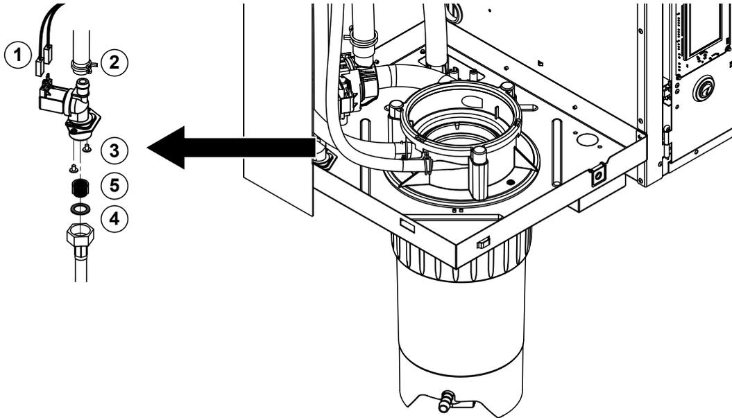
1. Detach electric cables (polarity of the cables must not be observed).
