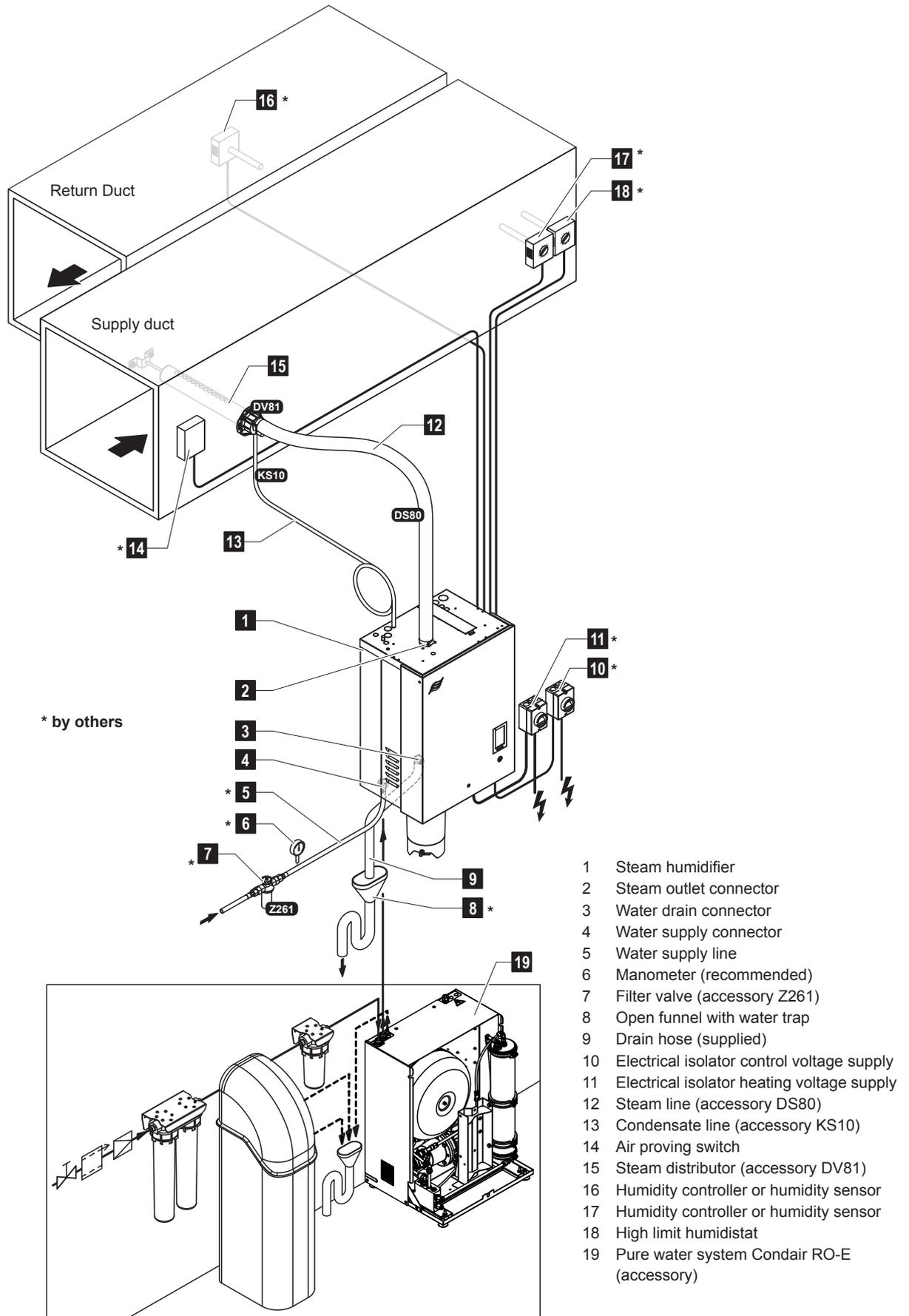
Fig. 2: System overview Condair RS for duct humidification
