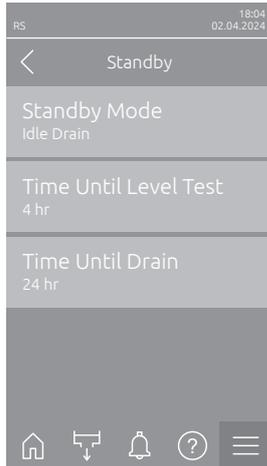
The following settings appear only, if "**Standby Mode**" is set to "**Idle Drain**".
