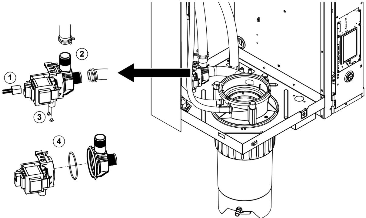
1. Detach electric cables (polarity of the cables must not be observed).
