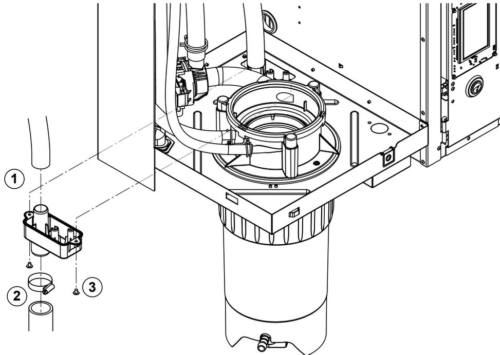
1. Remove drain hose from the connector on the drain cup.
