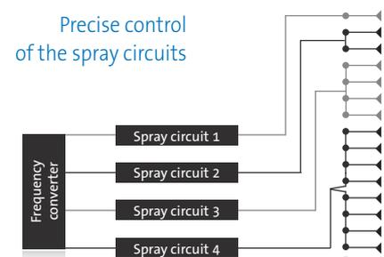
Precise humidifier output using frequency converters
